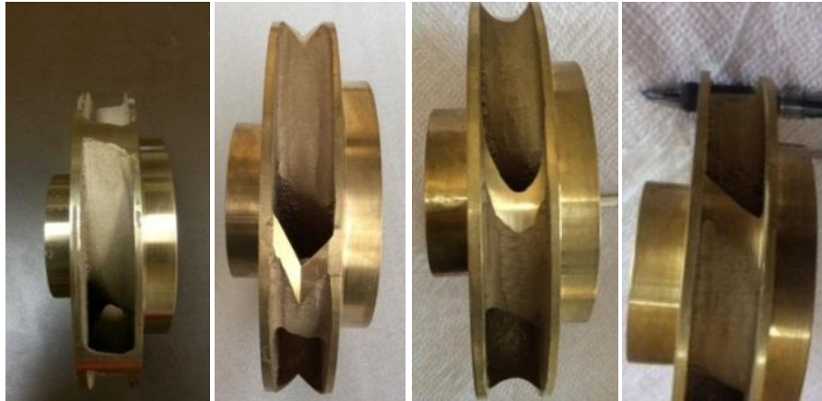
a. Impeller without blade cut b. Impeller with V-cut c. Impeller with C-cut d. Impeller with straight cut
